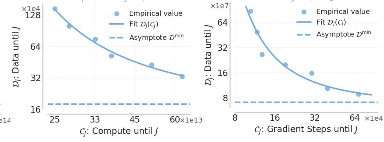
Each J corresponds to a  $\mathcal{D}$  –  $\mathcal{C}$  Pareto frontier. Each frontier has a unique budget-optimal point, corresponding to an optimal UTD\* and budget  ${\mathcal F}.$ Optimal UTD follows a power law wrt budget!
